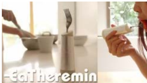
EaTheremin consists of a fork device, a micro controller (Arduino Uno), an audio board (MP3 TriggerBoard), and a speaker.
