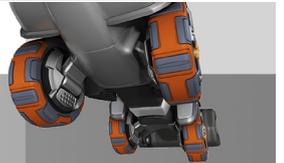
The independent suspension provides much greater maneuverability, less vibration and stability on the rough and uneven ground, thus offers a comfortable ride for operator. The articulated joint structure increases stability for both moving and standstill situations.
